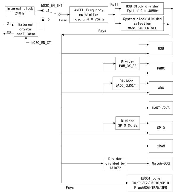
After selecting one of the two clocks, the internal clock or the external clock is used as the original clock Fosc, and then the Fpll high frequency clock is generated after PLL frequency doubling. finally, the system clock Fsys and the clock Fusb4x of the USB module are obtained through two groups of frequency dividers. The system clock Fsys is provided directly to each module of CH549.
